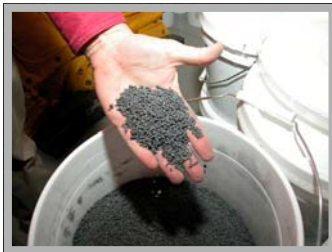
Ecomass® Material 2mm x 3mm Pellets
