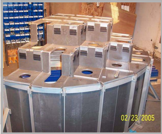
Reactor Vessel Head Shielding for Inspection / Repair
